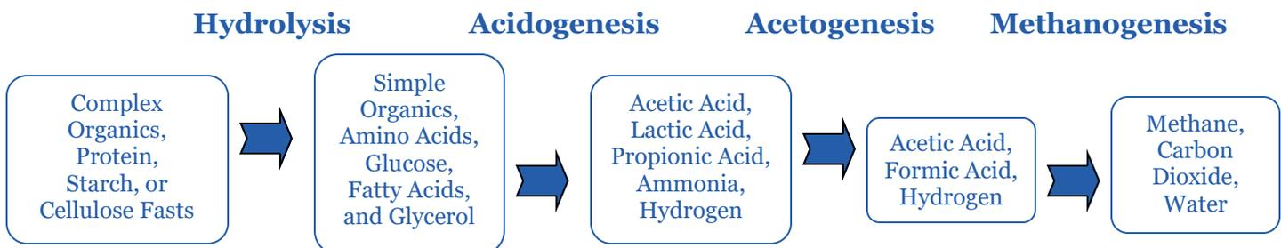
**Stage 1:** Hydrolysis converts complex polymeric organic compounds to simple compounds which can be absorbed and metabolized. Acidogenesis breaks these compounds down to volatile fatty acids, carbon dioxide and other low molecular weight compounds. Acetogenesis further converts a variety of simple metabolic products to acetic and formic acids and hydrogen.
